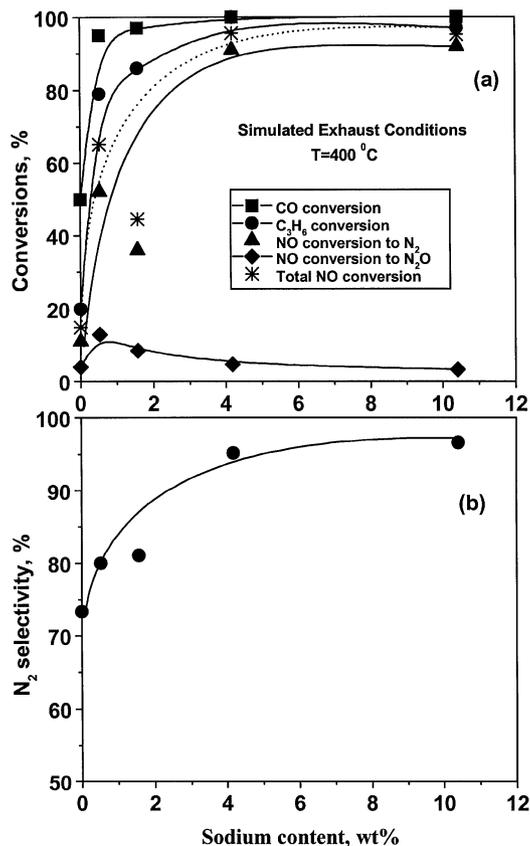
FIG. 5. The effect of sodium loading on reactant conversions (a) and selectivity towards  $N_2$  (b) for fixed temperature and inlet conditions. Data taken at  $400^\circ\text{C}$ , with a catalyst weight of 8 mg under simulated exhaust conditions (1000 ppm NO, 1067 ppm  $C_3H_6$ , 7000 ppm CO, and 7800 ppm  $O_2$ ). Total flow rate is  $80\text{ cm}^3\text{ min}^{-1}$ .
