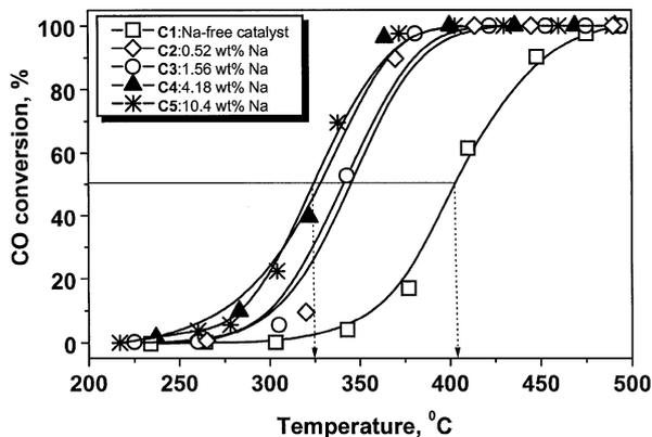
FIG. 2. Conversion of CO as a function of temperature for Pt/ $\gamma$ - $Al_2O_3$  catalysts with different sodium loadings. Data taken under simulated exhaust conditions at the stoichiometric point (1000 ppm NO, 1067 ppm  $C_3H_6$ , 7000 ppm CO, and 7800 ppm  $O_2$ ), with total flow rate  $80\text{ cm}^3\text{ min}^{-1}$ . Catalyst weight is 8 mg.
