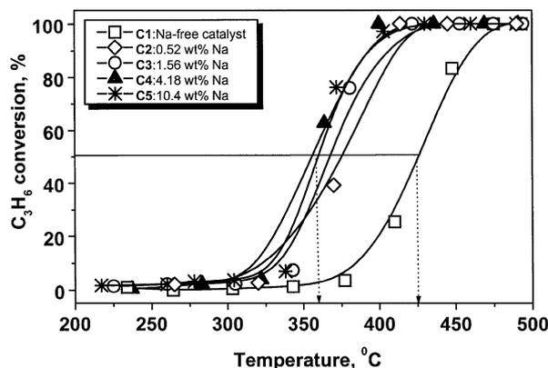
FIG. 1. Conversion of  $\text{C}_3\text{H}_6$  as a function of temperature for Pt/ $\gamma\text{-Al}_2\text{O}_3$  catalysts with different sodium loadings. Data taken under simulated exhaust conditions at the stoichiometric point (1000 ppm NO, 1067 ppm  $\text{C}_3\text{H}_6$ , 7000 ppm CO, and 7800 ppm  $\text{O}_2$ ), with total flow rate  $80\text{ cm}^3\text{ min}^{-1}$ . Catalyst weight is 8 mg.
