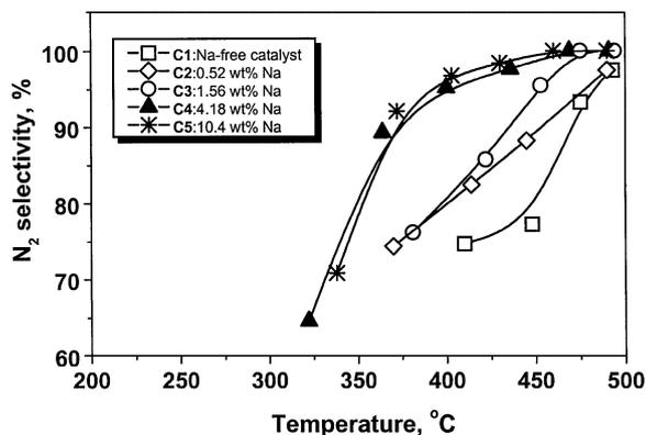
FIG. 4. Selectivity towards  $N_2$  as a function of temperature for  $Pt/\gamma\text{-Al}_2\text{O}_3$  catalysts with different sodium loadings. Data taken under simulated exhaust conditions at stoichiometric point (1000 ppm NO, 1067 ppm  $C_3H_6$ , 7000 ppm CO, and 7800 ppm  $O_2$ ), with total flow rate  $80\text{ cm}^3\text{ min}^{-1}$ . Catalyst weight is 8 mg.
