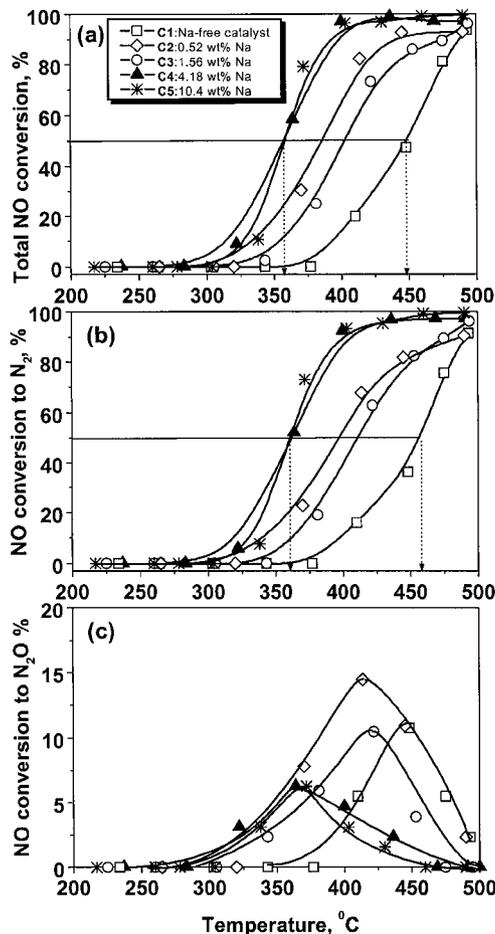
FIG. 3. The conversion of NO, (a) total, (b) to  $N_2$ , (c) to  $N_2O$ , as a function of temperature for Pt/ $\gamma$ - $Al_2O_3$  catalysts with different sodium loadings. Data taken under simulated exhaust conditions at the stoichiometric point (1000 ppm NO, 1067 ppm  $C_3H_6$ , 7000 ppm CO, and 7800 ppm  $O_2$ ), with total flow rate  $80\text{ cm}^3\text{ min}^{-1}$ . Catalyst weight is 8 mg.
