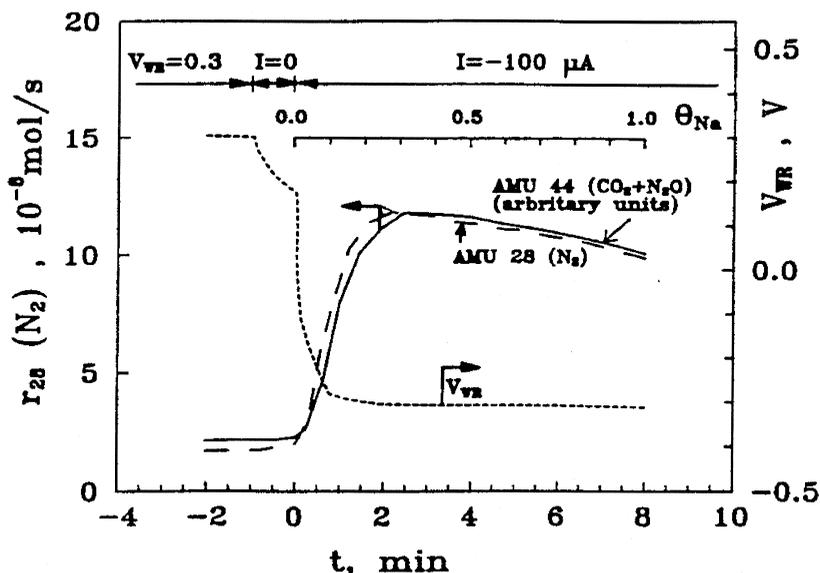
Fig. 2. Transient effect of applied constant negative current (Na supply to the catalyst) on the amu 28 ( $N_2$ ) and 44 ( $CO_2 + N_2O$ ) mass spectrometer signals and on the catalyst potential ( $V_{WR}$ ); conditions:  $p_{NO} = 1.3$  kPa,  $p_{C_3H_6} = 0.6$  kPa,  $T = 648$  K.
