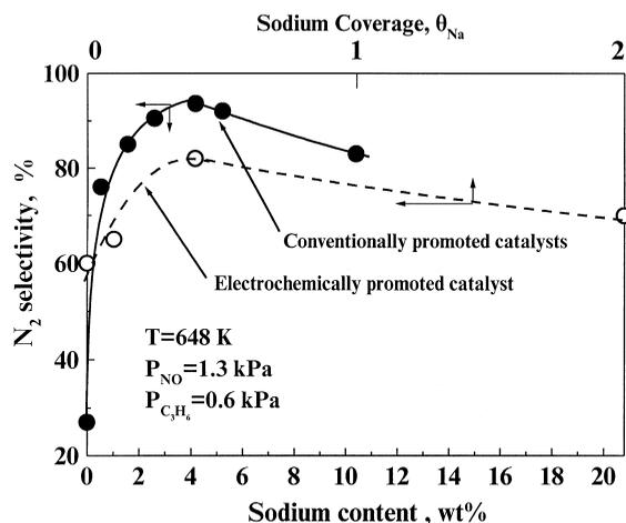
Fig. 4. Comparison of electrochemically promoted and conventionally promoted Pt at  $T=648\text{ K}$  with respect to N<sub>2</sub>-selectivity. Reactor inlet conditions:  $p_{NO}=1.3\text{ kPa}$ ,  $p_{C_3H_6}=0.6\text{ kPa}$ .
