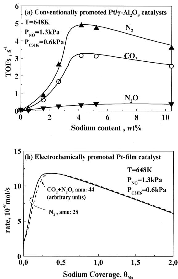
Fig. 3. Comparison of EP and conventional promotion data at  $T=648\text{ K}$  taken under similar reactor inlet conditions:  $p_{NO}=1.3\text{ kPa}$ ,  $p_{C_3H_6}=0.6\text{ kPa}$ . (a) Conventionally promoted Pt/ $\gamma$ -Al<sub>2</sub>O<sub>3</sub> catalysts, (b) electrochemically promoted Pt-film catalyst using the transient galvanostatic mode of operation.
