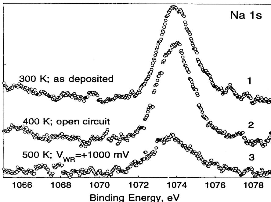
Fig. 1. Na1s XPS illustrating electrochemical pumping of vacuum-deposited Na away from the surface under UHV conditions at sufficiently high temperature and positive catalyst potential.
